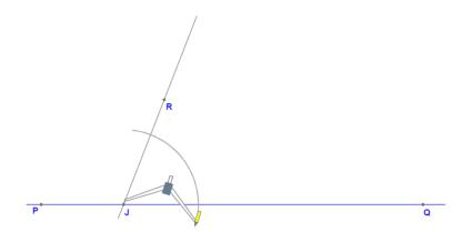
3. Using the same distance on the compass, construct a copy of the angle formed by the transversal at point R
