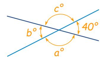
Because b° is vertically opposite 40°, it must also be 40° A full circle is 360°, so that leaves  $360^\circ - 2 \times 40^\circ = 280^\circ$ Angles a° and c° are also vertically opposite angles, so must be equal, which means they are 140° each.
